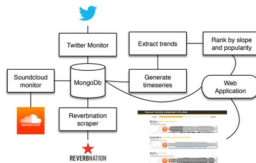
Figure 1. Diagram of the discovery system.
